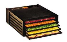
Excalibur manufactures a horizontal air-flow dehydrator with the heating element and fan located at the back of the unit. The major advantages of horizontal flow are: it reduces flavor mixture so several different foods can be dried at one time; all trays receive equal heat penetration; and juices or liquids do not drip down into the heating element. These units are not widely available.
