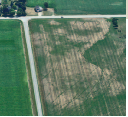
This summer aerial view makes bedrock cracks obvious. In places like this, extra care is needed to prevent surface pollution from entering groundwater.
